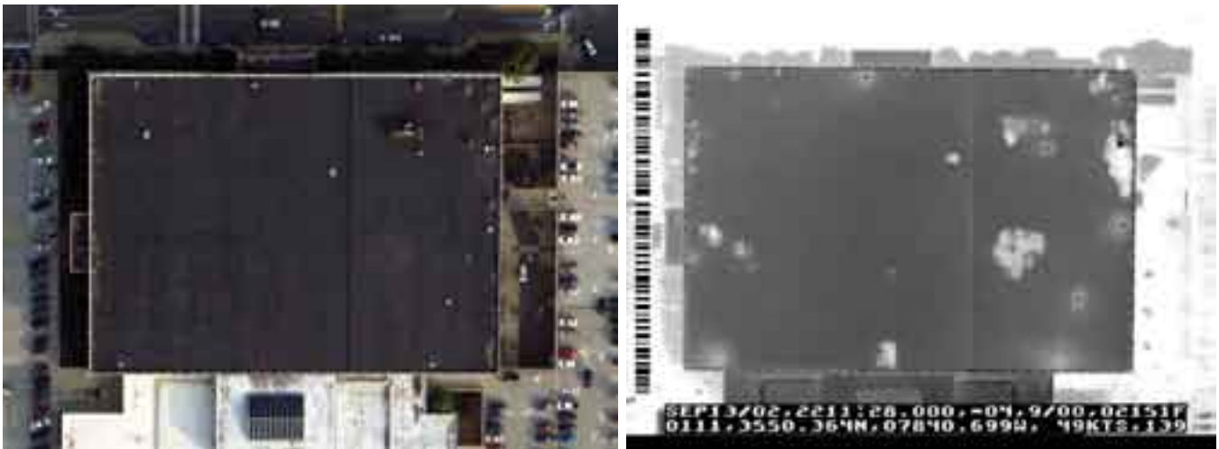
TWO VIEWS Infrared imaging (right) can reveal problem spots on roofs not normally visible to the naked eye (left).
